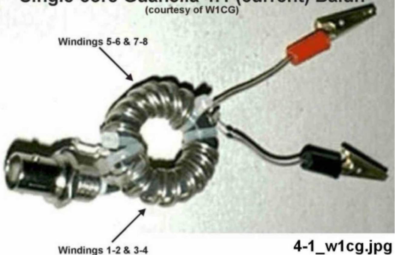
Label the 7-8 lead as RED (colors correspond to the approximate colors of the wires used in the R/S #24 speaker wire (278-1509), label the 5-6 lead as White, 3-3 as RED and 1-2 as WHITE.
